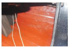
This area of deck beam is at critical stage aft left behind main cabin 50% is gone It has not yet been taken out due to wanting to make this wood first
